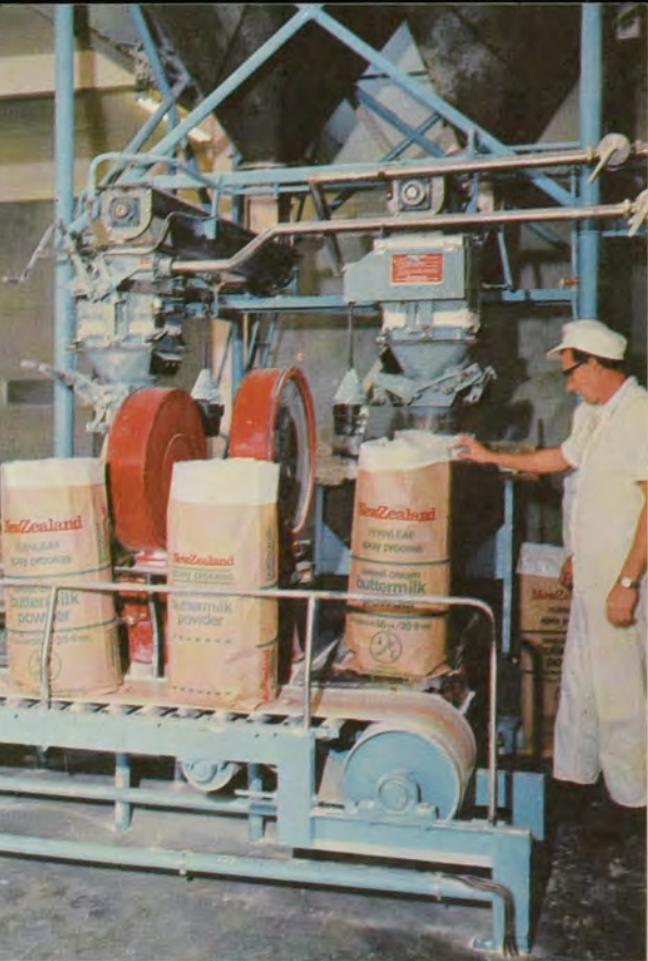
ABOVE Inside a New Zealand Milk Powder manufacturing plant, showing multiwall bags beneath the filling hoppers.
